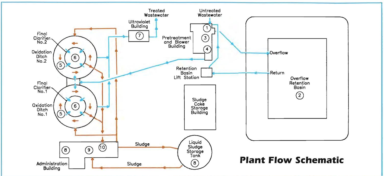
**5) Oxidation Ditches:** Biological treatment of the wastewater takes place in the two oxidation ditches. Raw wastewater is mixed with microorganisms that feed on bacteria and organic material. The microorganisms clump together to form a biological floc. Air and alum, a chemical that reduces phosphorus in wastewater, are added to the process at this point.
